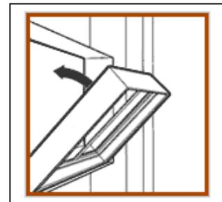
or bottom of the frame surfaces as this could cause leakage during a rain storm. **Note:** Pilot holes should be drilled through the vinyl window frame and shims to prevent cracking of the vinyl frame and shims.
