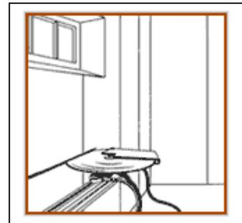
After cutting the **Poured Concrete Wall** on both sides break-out with a 3-pound hammer, clean up cut surfaces if necessary using a cold chisel and 3-pound hammer. Go to Step 4:
